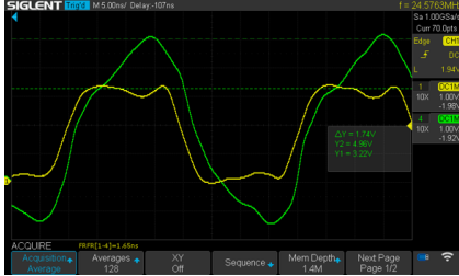
Figure 2: Input (yellow) and output (green) signals of one of the buffers with measured delay of 1.65 ns.
